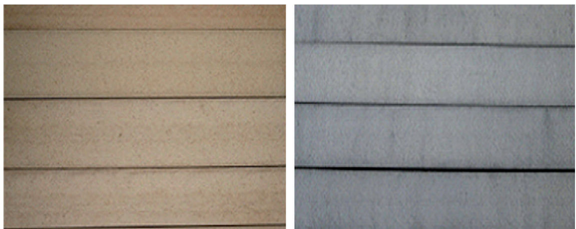
Figure 9. Photos of HDPE-based WPCs before and after natural weathering [23].
