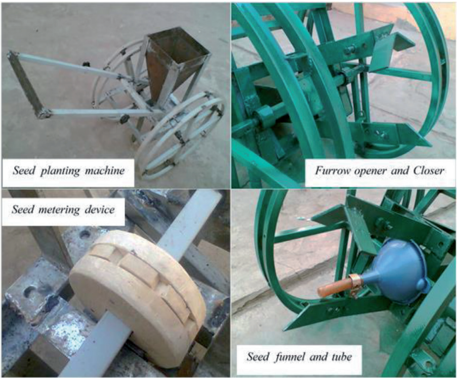
Figure 3. Component parts of the maize planter. Source: [16].
