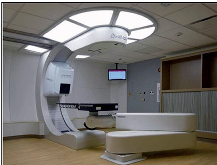
Figure 1. Single gantry radiation therapy system. Copyright. Creative commons attribution license (CC BY) [16].
