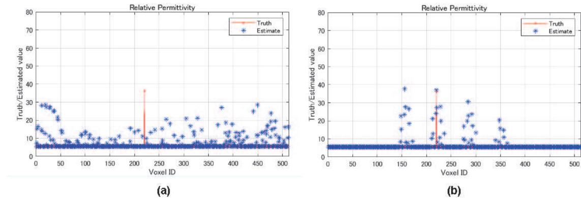
**Figure 14.** (a) Reconstructed relative permittivity (resolution of 5 mm, printed dipole is used). (b) Reconstructed relative permittivity (resolution of 5 mm, FQSCA is used).
