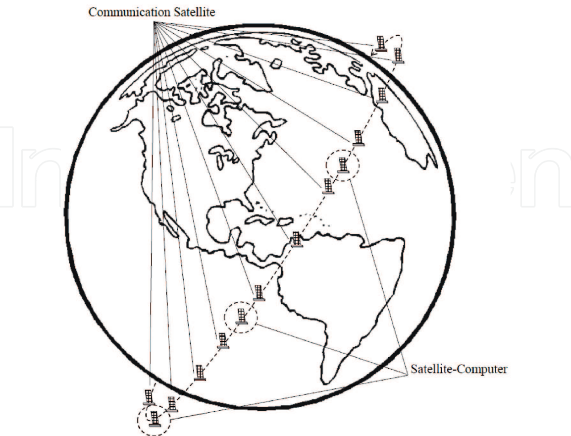
Figure 7. Location of satellites-computers in one orbital plane of the StarLink constellation.
