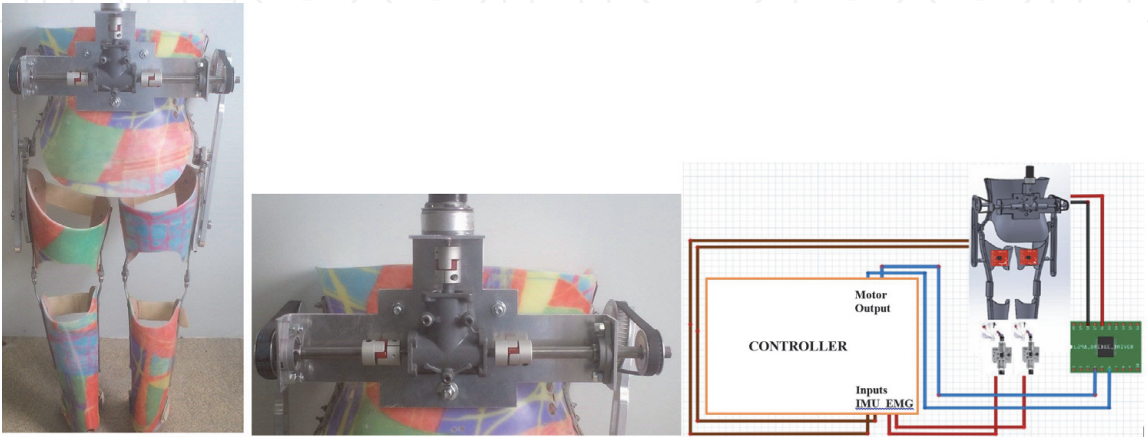
Figure 12. Hip-knee-ankle-foot-orthosis (HKAFO): (A) system configuration, with T-type deflector reducer; (B) control circuit (online video: [98]).
