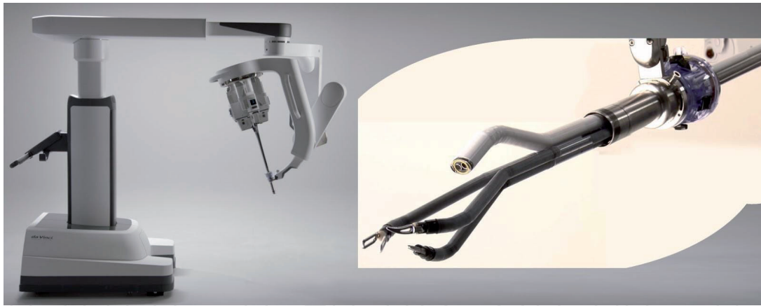
Figure 3. Single channel robotic arm with multiple instruments.
