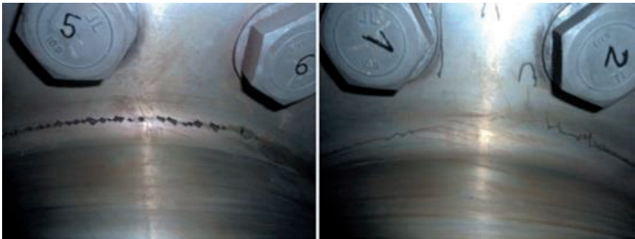
Figure 2. Fracture of hoist’s shaft [8].
