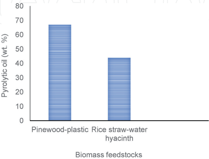
Figure 7. Pyrolytic oil generation from biomass co-pyrolysis process at 400 °C [9, 42].
