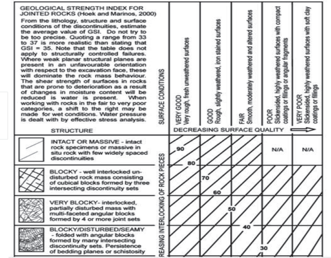
Figure 5. Geological strength index chart [15].
