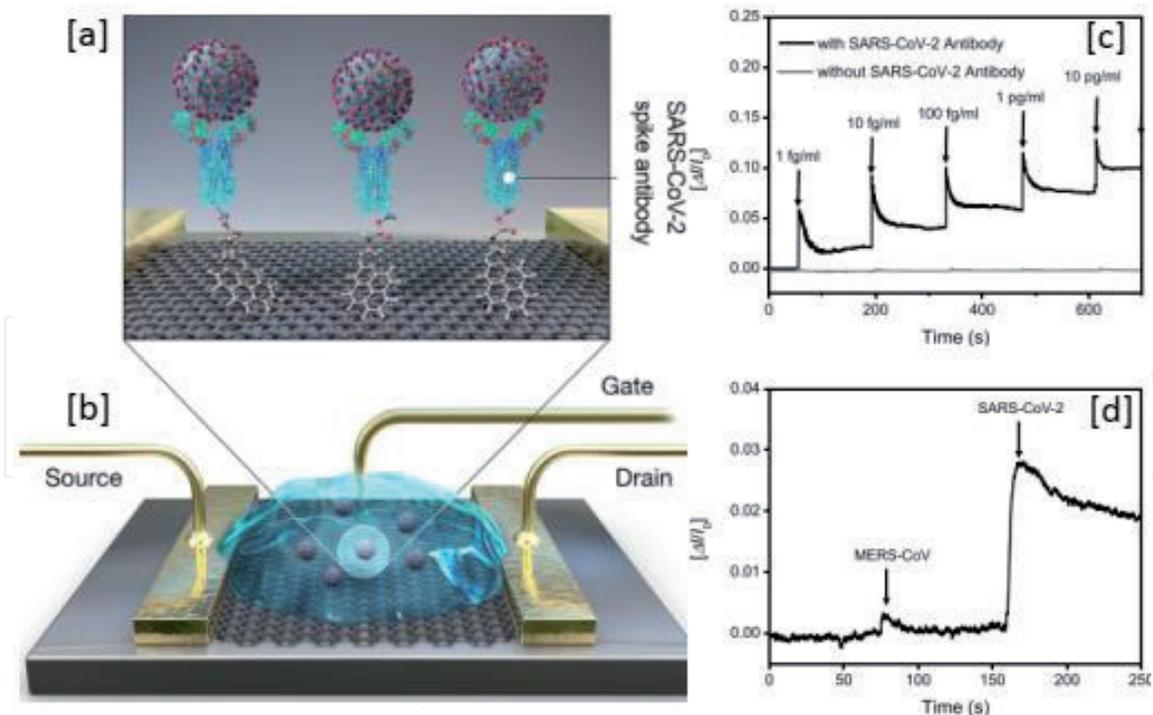
**Figure 6.** (a) showing conjugation of spike protein on to the surface of graphene via 1-pyrenebutyric acid *N*-hydroxysuccinimide ester (b) model showing spike protein on the surface (covered with graphene) of field effect transistor (c) FET sensor sensitivity in presence of SARS-COV-2 antibody and in absence of SARS-COV-2 antibody and (d) FET sensor sensitivity in MERS-COV and SARS-COV-2 (reproduce with permission [32]).
