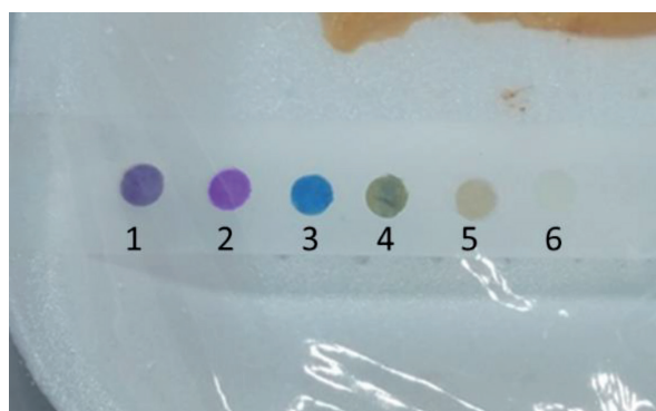
Figure 4. An example of the array placed over the tray containing the poultry meat, with sensors from one to six based on m -cresol purple (1), o -cresol red (2), bromothymol blue (3), thymol blue (4), chlorophenol red (5), and the Ellman's reagent (6).
