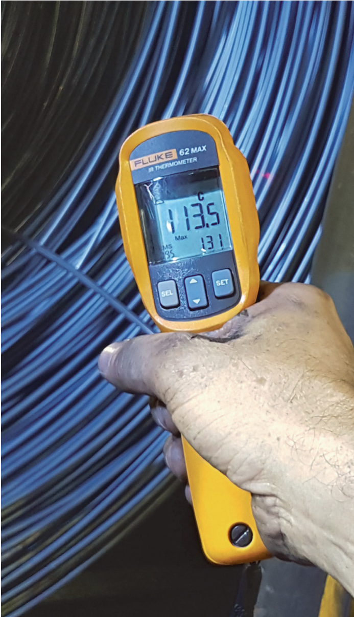
Figure 5. Coil temperature at the hot rolling process outlet at 113.5°C.
