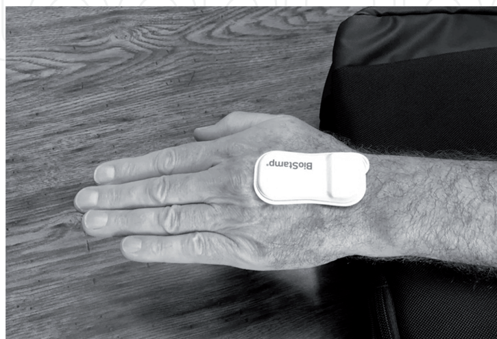
Figure 8. The BioStamp nPoint conformal wearable and wireless inertial sensor system mounted about the dorsum of the hand for quantifying movement disorder tremor response, such as for Parkinson's disease, as a result of deep brain stimulation intervention [112].
