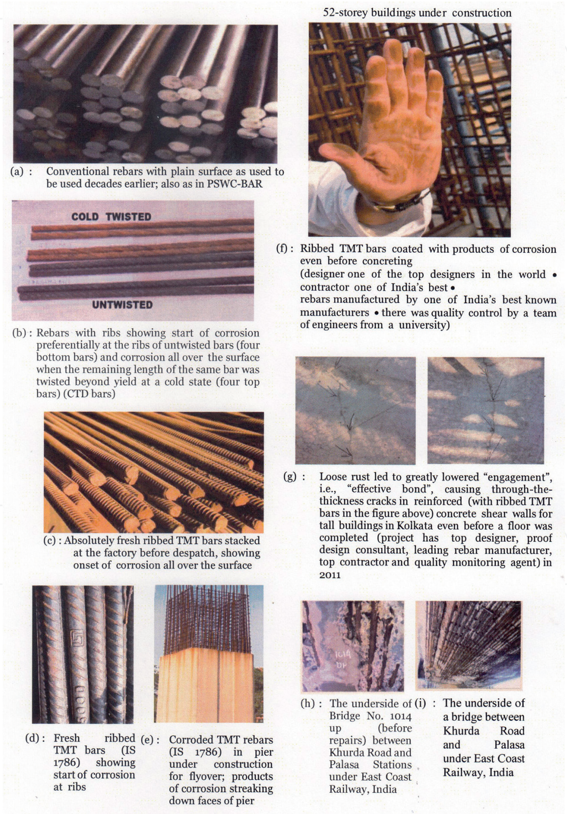
Figure 6. A collection of plain bars free from rust and ribbed CTD and TMT bars with various stages of corrosion.
