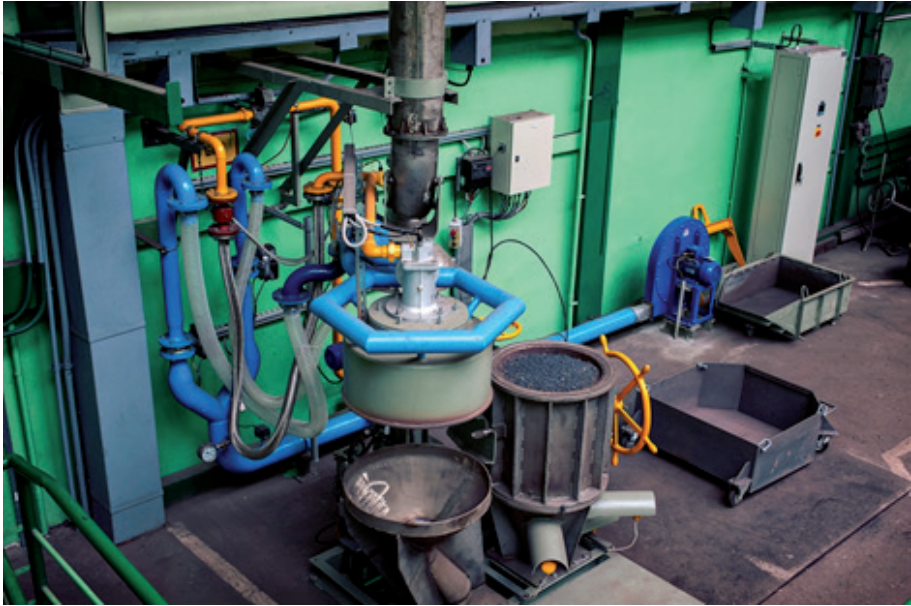
Figure 2. The experimental site for sintering iron ores and waste products in Sieć Badawcza Łukasiewicz - Instytut Metalurgii Żelaza.
