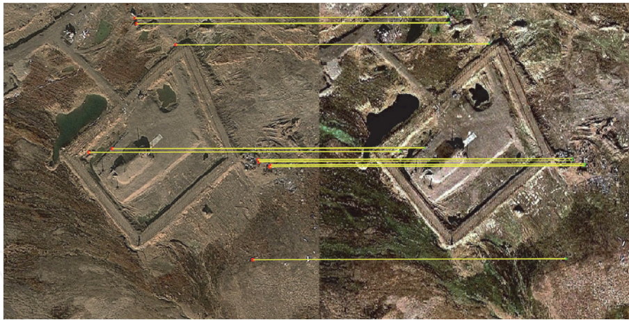
Figure 5. Image pair (I_0, I_1) matching result for ORB method.
