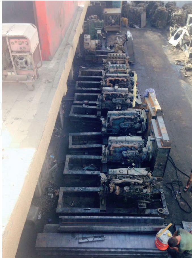
Figure 3. Assembly line of a local manufacturer of neighbourhood diesel generators (Source: Local assembler).
