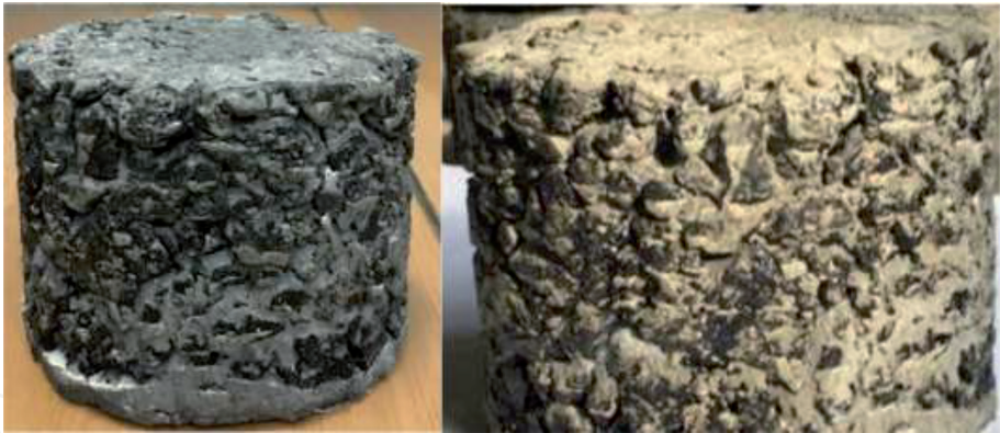
Figure 2. Disconnectivity of internal voids due to low air-voids [18].
