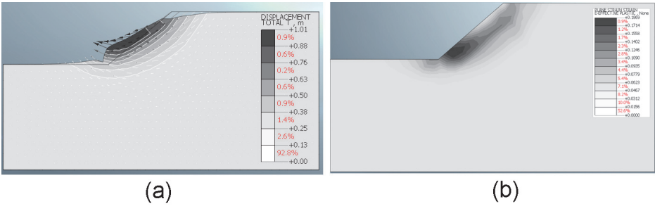
Figure 6. Distribution of displacement and shear strain by finite element analysis under slope failure condition (case 1).
