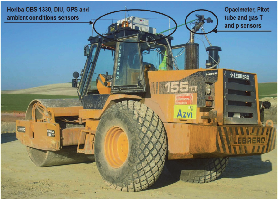
Figure 7. View of the experimental installation located on the construction machine.
