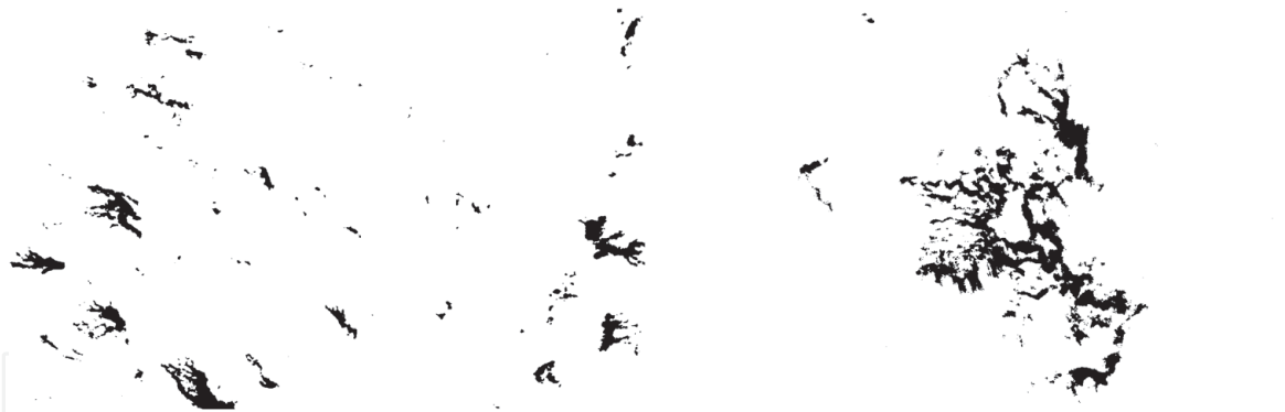
Figure 14. Morphologies of linear (left) and feathery (right) shrinkage porosity.
