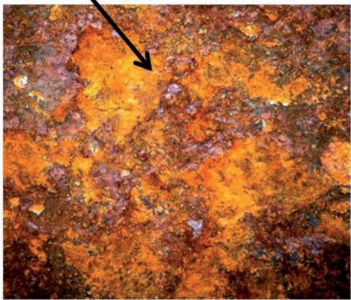
Figure 9. Corrosive and oxidation wear of structural members of industries.
