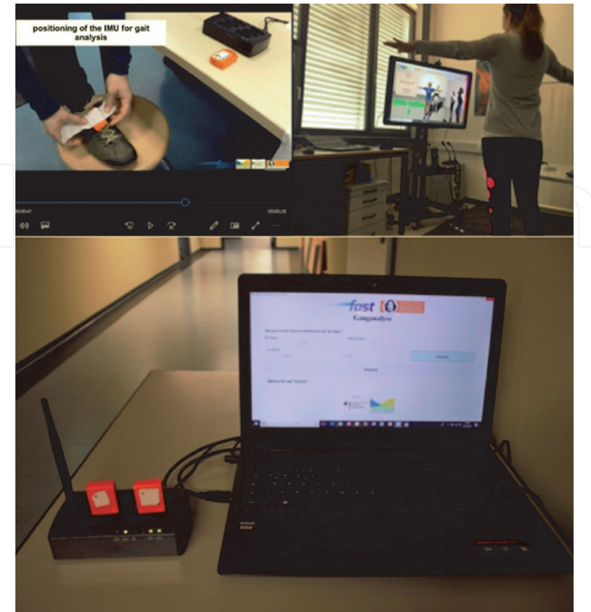
Figure 7. Setup of the gait measurements for e-rehabilitation of Otto von Guericke university; above left: IMU application at the feet; above right: Therapeutic movements with avatar; lower middle: Presentation of gait analysis measurement.
