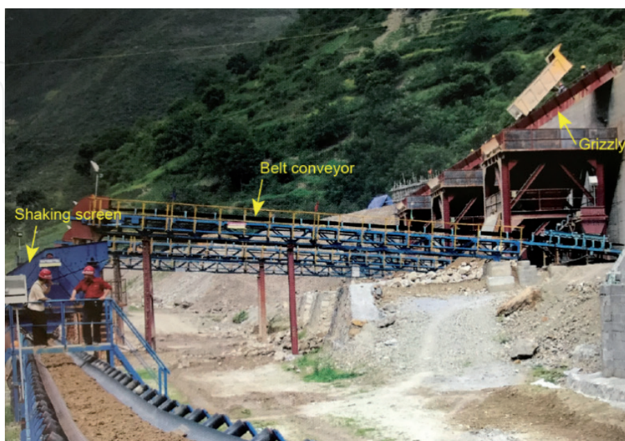
Figure 14. Screening system for the PBG dam (at the courtesy of Yao FH).
