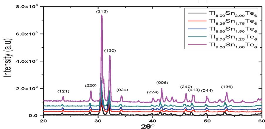
**Figure 4.** X-ray diffractometry of  $Tl_{10-x}Sn_xTe_6$  doping Sn = 1, 1.25, 1.50, 1.75 and 2.
