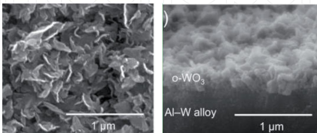
**Figure 10.** SEM images of the surface and cross-sectional of WO<sub>3</sub>. Reproduced by Higashino et al. [103].
