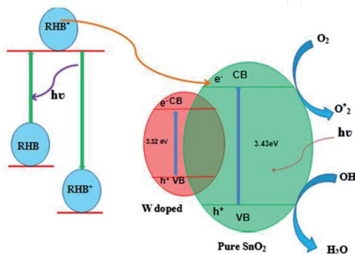
**Figure 12.** Schematic representation for photocatalytic mechanism of RHB in W-SnO<sub>2</sub> thin films. Reproduced by Vadivel et al. [120].
