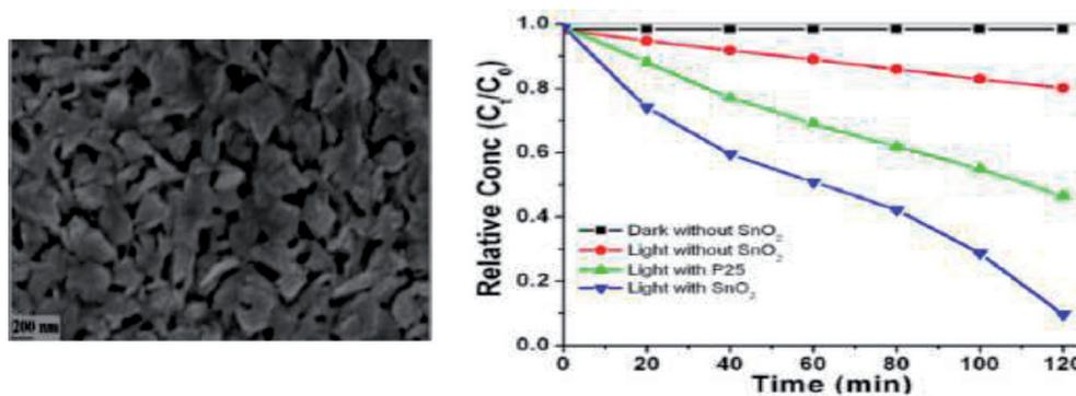
**Figure 11.** The SnO<sub>2</sub> thin film and the photocatalytic activity of SnO<sub>2</sub> thin film. Reproduced by Jana et al. [112].
