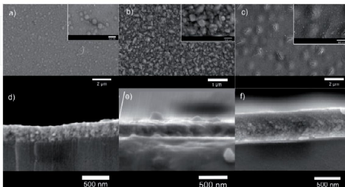
**Figure 9.** SEM images of the (a)  $\text{ZrO}_2$ , (b)  $\text{TiO}_2$  and (c)  $\text{ZrO}_2\text{-TiO}_2$  composite films with the high magnification. The side on images—(d)  $\text{ZrO}_2$ , (e)  $\text{TiO}_2$ , and (f)  $\text{ZrO}_2\text{-TiO}_2$  composite—shows the film thickness. Reproduced by Alotaibi et al. [32].
