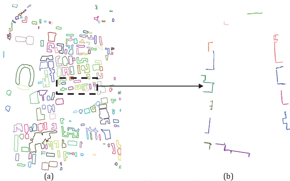
Figure 7. Illustration of building boundary extraction results from (a) over-view and (b) ground-view data.
