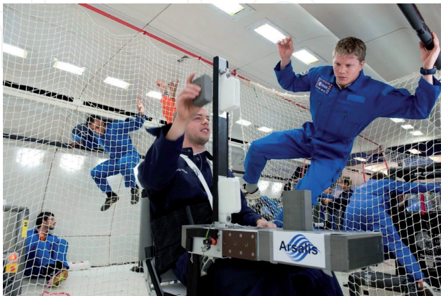
Figure 4. Test of the GRIP restraint system using a GRIP mock-up chair during the 53rd ESA parabolic flight campaign of October 2010 (photo: ESA).
