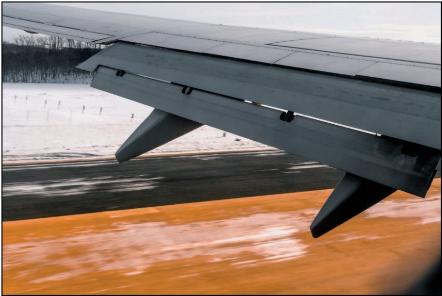
Figure 7. Wing with extended flaps.
