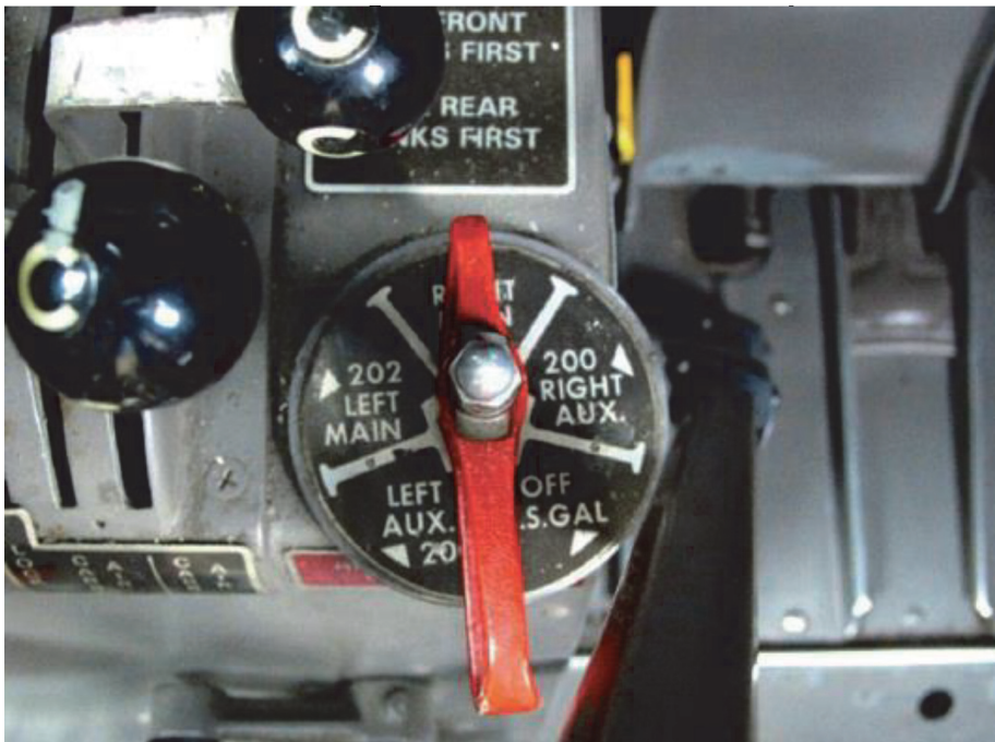
Figure 13. Fuel valve with detents and the indicating handle for each position.
