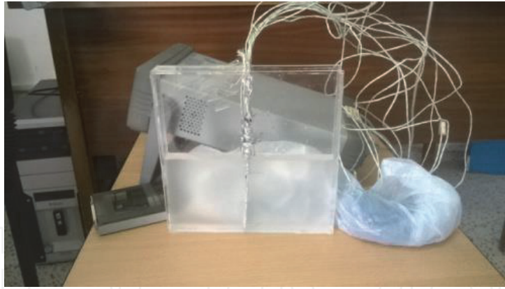
Figure 2. PCM wall filled with Paraffin-27.
