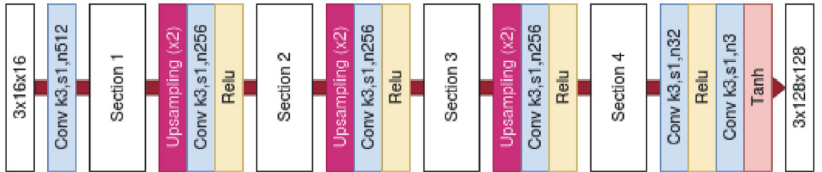
Figure 14. Architecture of the low to high generator.
