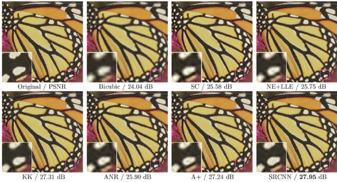
Figure 4. Comparisons between [7] and state-of-the-art model based methods.
