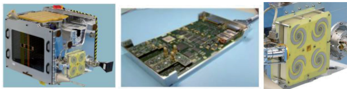
Figure 10. (Left) TechDemoSat-1 (TDS-1) prior to launch (Centre) SGR-ReSI, part of sea-state payload on TDS-1 (Right) TDS-1 nadir GNSS antenna [14].
