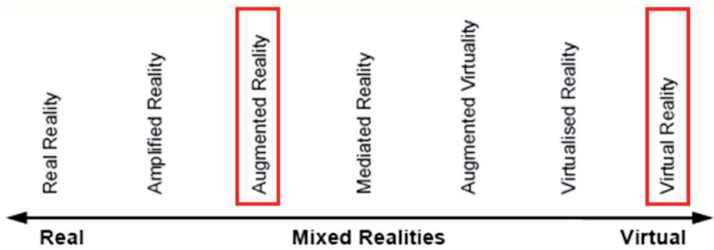
Figure 1. Order of reality concepts ranging from reality to virtuality (Schnabel et al., 2008) [4].
