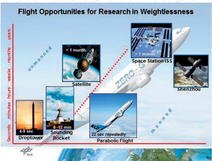
Figure 9. Reduced gravity platforms accessible to microgravity researchers (vertical axis, duration of microgravity; horizontal axis, quality of microgravity) (credit: DLR).
