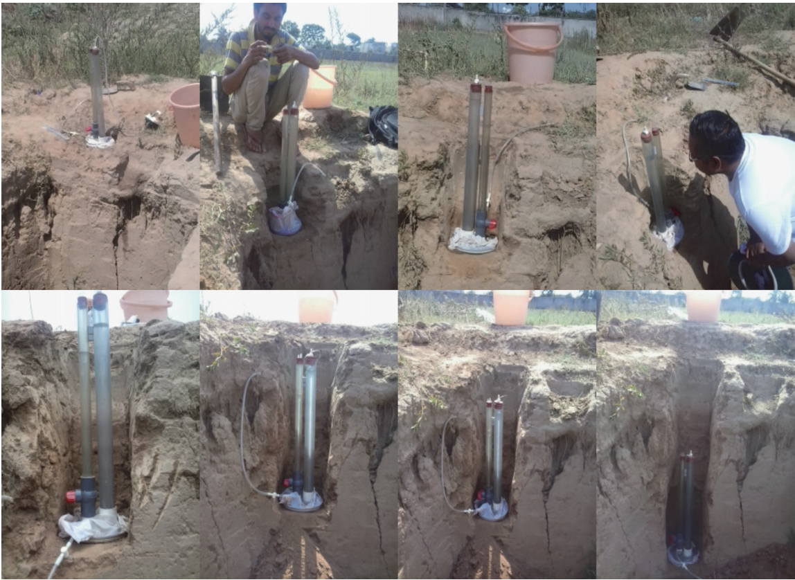
Figure 11. Disk permeameter for delineation of un-saturated hydraulic conductivity [23].
