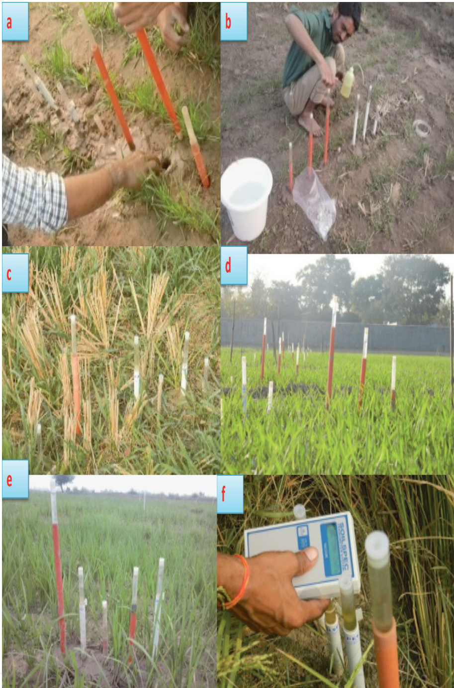
Figure 10. Working of electronic tensiometers (a) Fitting of tensiometers in the field, (b) filling of water in tensiometers, (c–e) installed tensiometers, (f) measuring of matric potential using digital soil spec [24].
