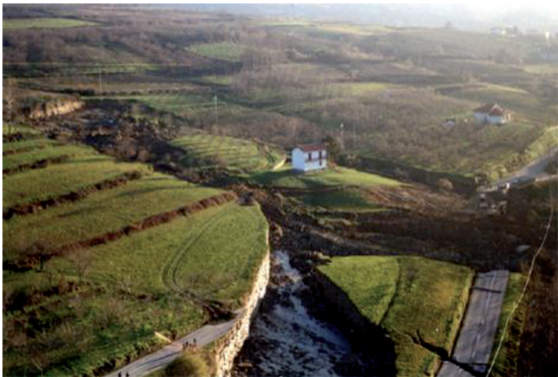
Figure 11. Rock-block slide near Feisoglio town: The mass movement slid about 50–60 m from their original position, destroying a road. The estimated area was about 4.63 ha, while the volume was about 385,000 m³. The gray layer surface is evident. The small white house moved together with the rock block nearly undamaged.
