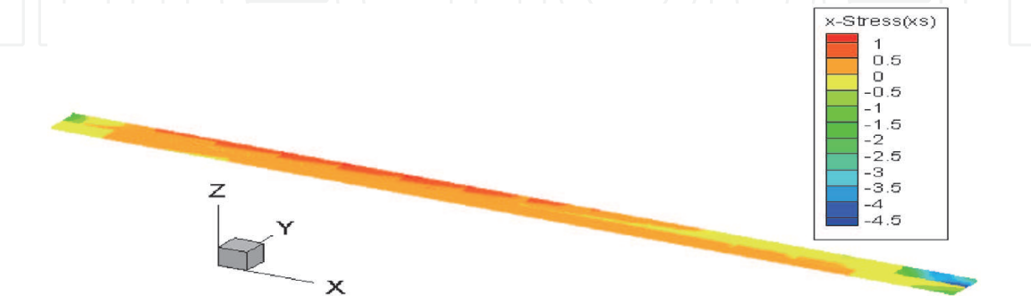
Figure 15. Contour of the dam axial stresses of the connecting plate and toe slab during the storage period (MPa).
