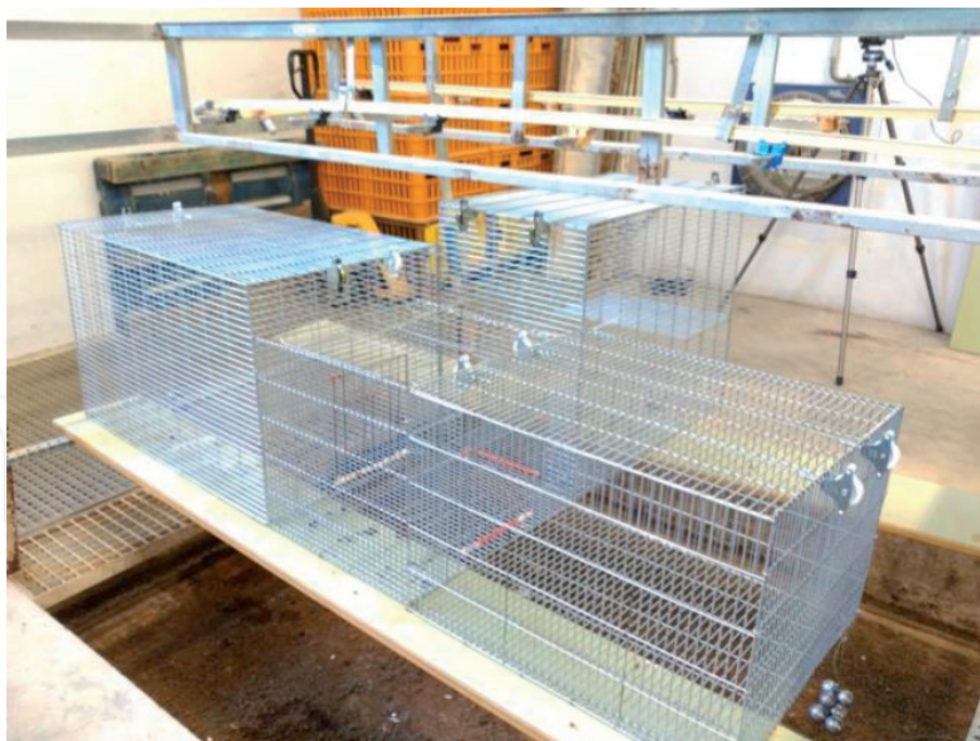
Figure 1. Motivation cage constructed to assess the preference of breeding does for different sizes of cages.
