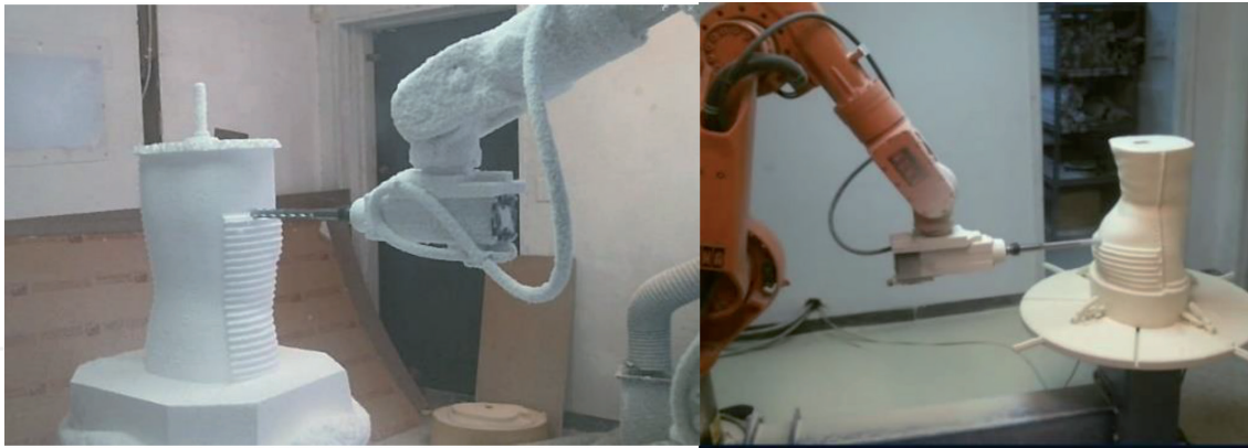
Figure 9. Robot-assisted spinal orthosis molds production.
