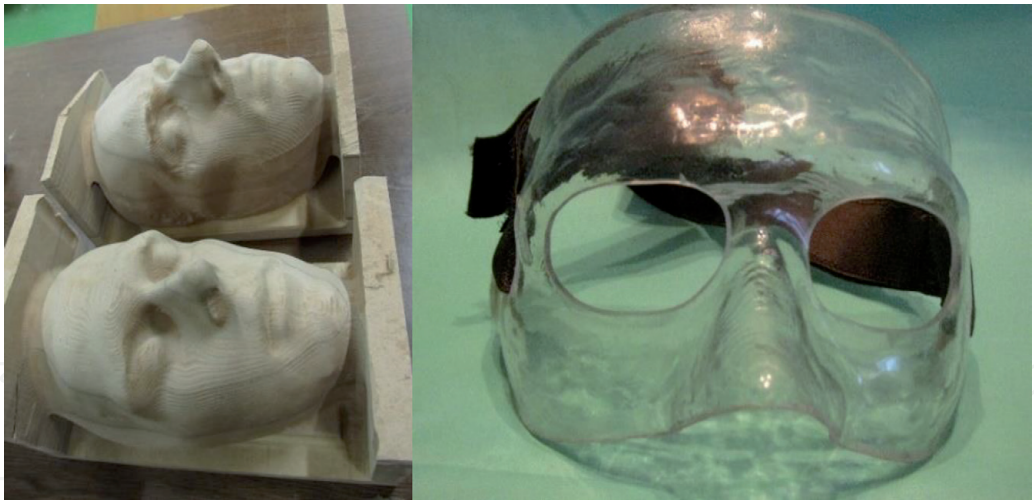
Figure 14. Molds made on three-axis milling machine and custom protective facial mask.
