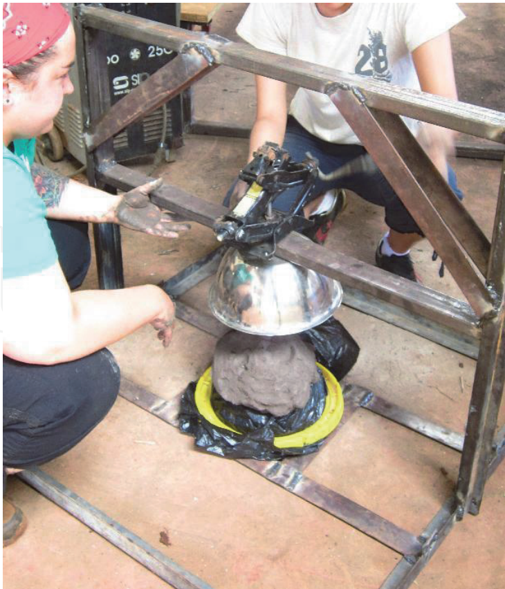
Figure 3. A low-cost filter press prototype [10].
