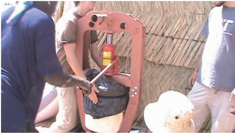
Figure 5. Operating the portable Pfp press with crank system [15].
