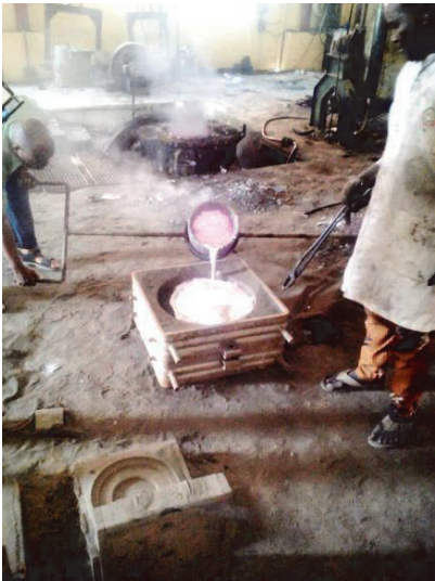
Figure 19. Pouring in the molten metal into the sand mould using furnace tongs.
