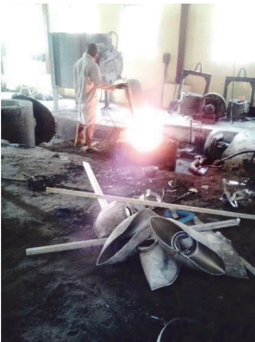
Figure 15. Process of melting the scrap aluminium in a rotary furnace.
