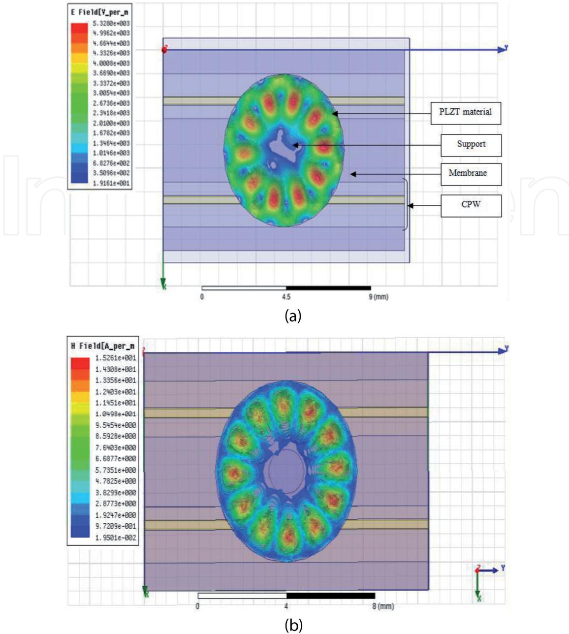
**Figure 10.** Amplitude of the magnetic field of the gallery modes: (a)  $WGH_{6,0,0}$  and (b)  $WGE_{5,0,0}$ .
