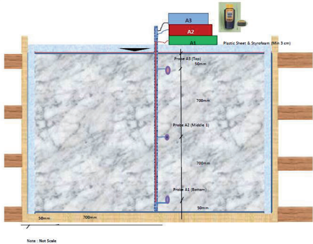
Figure 20. Thermocouple Fc'25 concrete+20%FA + ice, monitoring, Summary Data & Mock up Sketch.
