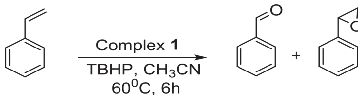
Figure 14. Oxidation of styrene using [\text{Ni}(\text{L}^1)(\text{NCS})_2] as catalyst.
