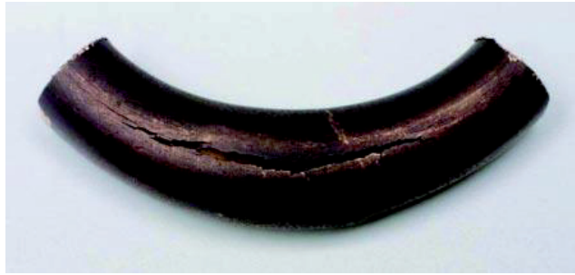
Figure 12. Macroscopic image cracked copper tube.
