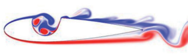
Figure 12. The vorticity contour plot over the airfoil with a cavity [63].
