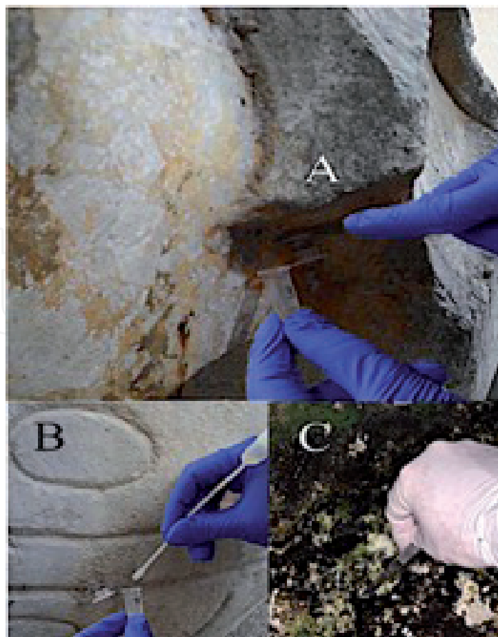
Figure 1. Stonework altered areas, sampling performed by sterile swab o scalpel: (A) dark-rust red area; (B) light – green calcareous deposit; (C) dark-green area.
