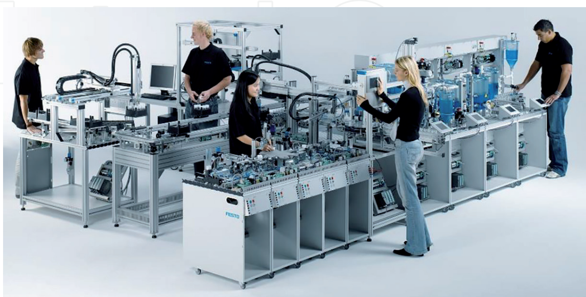
Figure 4. An example of an FMS developed by FESTO group.
