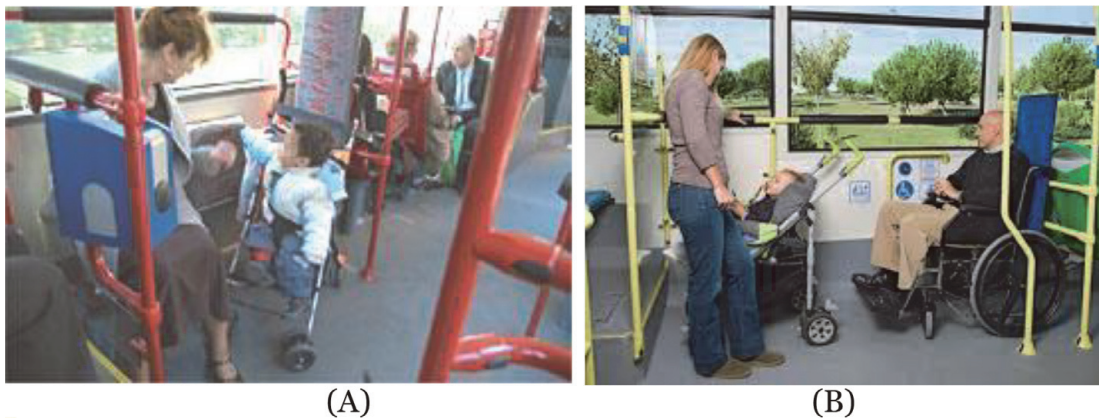
Figure 2. Examples of the safety conditions in the mobility of ChC in passenger public transportation vehicles: (A) absence of safety systems to hold the ChC unfolded during travel, (B) compatibility of ChC with the WHCHs' space occupied (source: EMT Madrid).
