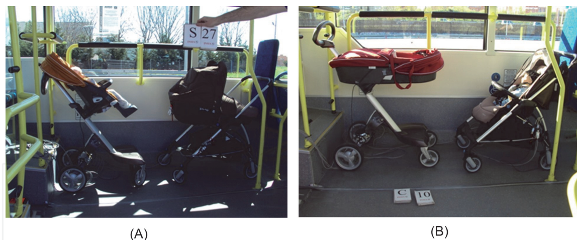
Figure 6. Provision of ChC deployed during experimental open circuit trials: (A) unfolded rearwards facing Model A carriage and forwards facing Model C carriage; (B) unfolded rearwards facing Model B carriage and forwards facing Model C carriage (source: [14])
